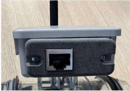
1/ Select the RJ45 connection On the lateral side of the electrical box
