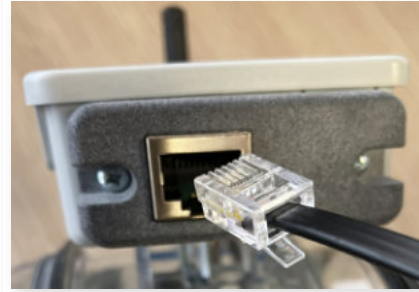
2/ Plug the cable delivered with the e-VAV
